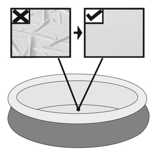
Put 1" to 2" water in the pool to cover the floor. Once pool floor is slightly covered, gently smooth out all wrinkles. Start in the center of the pool and work your way clockwise to the outside.
