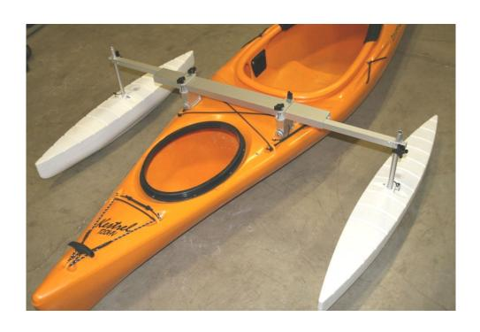
3. Once the proper location is determined mark and drill the holes for the brackets using a 1/4" drill bit.
