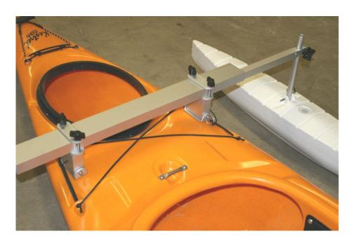
6. Attach support bar to the canoe using the angle brackets and the long u-bolts. The long side of the angle should be towards the canoe interior. It may be possible to use these same brackets to attach the
